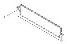
1 securing clip (snapped in position)
